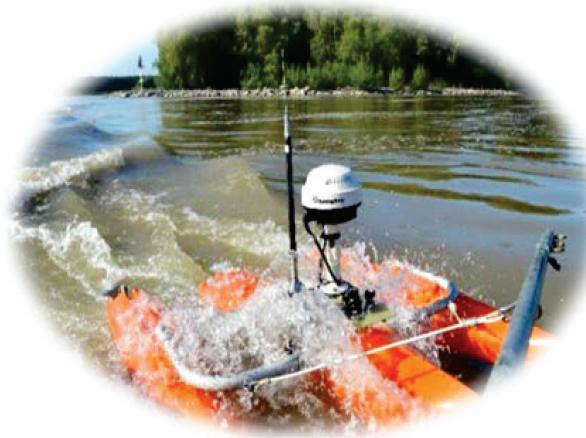
RiverRay ADCP for flow-speed measurement
