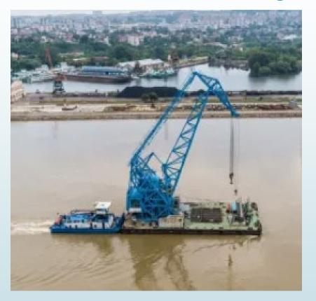
Vessel 'Titan' – 100 ton floating crane
