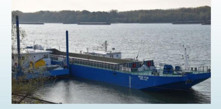
Non-self-propelled hopper barge NSPS 1139
