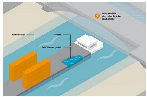
Figure 4: Drawing of the demolition vessel "Killian". Source: ASFINAG.
