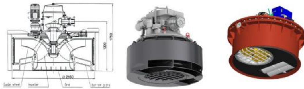
Figure 29: Schottel Pump-Jet and Veth's Compact-Jet. Source: Radojčić et al. (2021).
