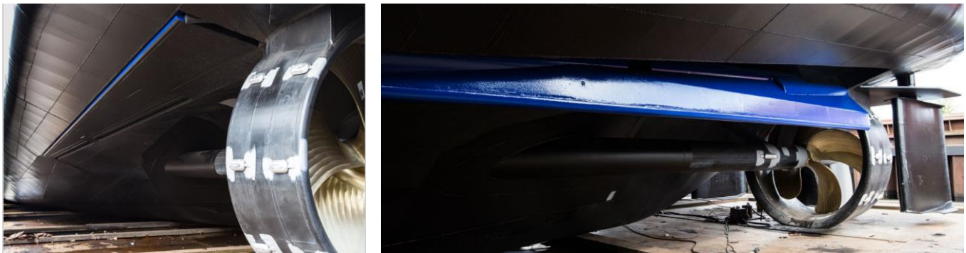
Figure 32: Flex Tunnel of Van der Velden. Left: retracted into the hull if the ship. Right: extracted for operation with small draught at low water depths. Source: Damen 10
